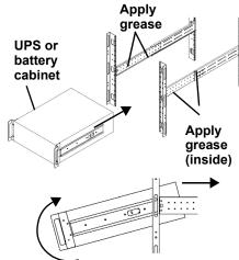
Insert the UPS into the front members, lift the front and push it into the rack.
